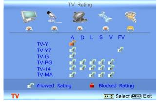
Press the **T** or **S** button to navigate through the TV rating options. Press the **D** button to block (locked) or allow (unlocked).
